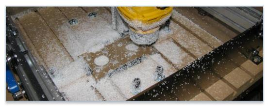
Your project may need some finishing touches, such a sanding, routing, cutting, or millwork. Projects can be carved more than once, so don't be afraid to layer your design. When you are finished carving on your material, remove the bolts, clamps, step blocks, and Smart Clamp to release your project. Please remember place everything back in its container, including the endmill and vacuum up the mess made by the X-Carve.
