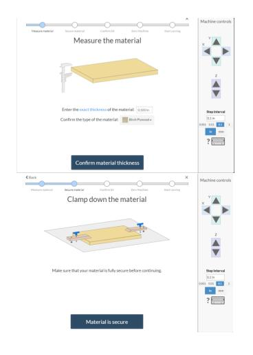
There are five steps to start your project. The first three steps just confirm that your material is of the right dimensions, your material is firmly fixed in position and that you have the appropriate bit size. Failure to verify any of these steps can lead to a depth error, ruined material, and gaps in your design.
