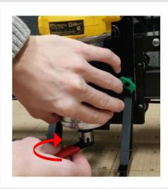
TIGHTEN THE COLLET TO THE SPINDLE WITH WRENCHES
