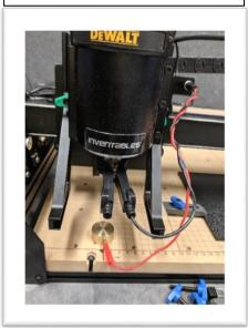
Z probe fully attached with clip
