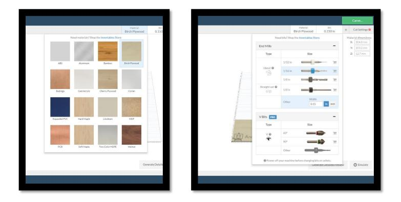
**\*Tips and Tricks:** thinner materials (1/8") tend to be pulled upward because of the cutting force of the X-Carve. Think about using a downcut endmill, using a sacrifice board to protect the wasteboard, and ask if you would be able to tape the material down. The Creative Space Support Associate or the Computer Desk Staff should tell you whether that would be appropriate for your material.
