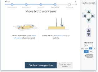
This step will only appear if you selected that you did not have a Z probe. If you elected to use the Z probe, you zero the machine by lowering the bit to touch the probe as it sits above the material.
