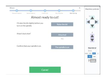
The last step will raise the bit so that it's not against the material. You should then confirm if you are going to use the dust shoe as the machine runs, and then turn on the spindle by hitting the power button on the side of the DeWalt 611.
